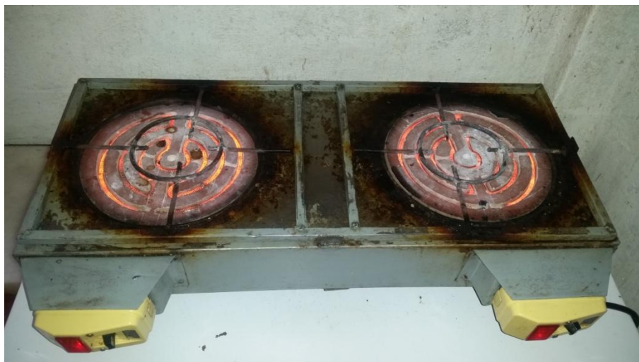
Figure 20. A stove's cook pot rest eccentric to the heating element
