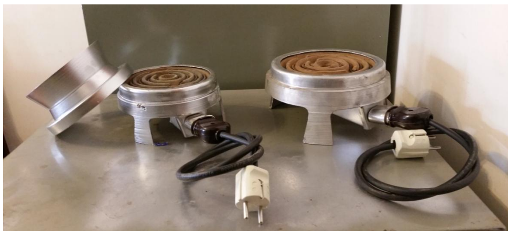
Figure 24. Lejo Aluminium Plc, Addis ababa, Ethiopia, stamped Aluminum body electric Stoves
