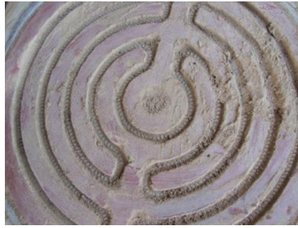
Figure 12. Clay plate of locally manufactured electric stove sealed using clay material
