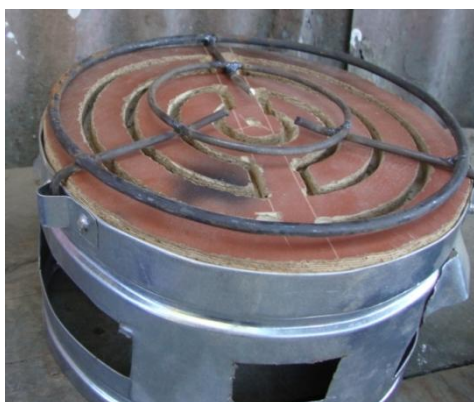
Figure 18. Groove and gap of cooking pot rest on local stoves.
