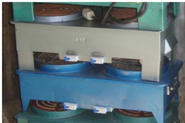
Figure 19. Local stoves made with circuit breakers instead of switches.
