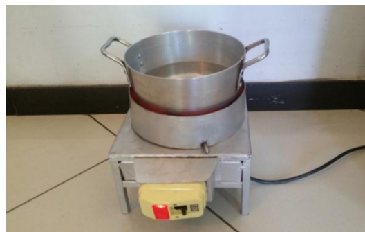
Figure 11. Double and Single stoves having bottom insulation and top lateral heat retainers
