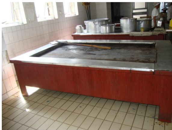
Figure 13. Locally manufactured “Karenbola” type electric stoves for large kitchens, 21 Kw
