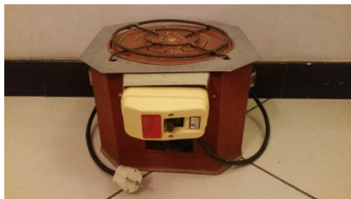
Figure 6. 18 cm and 22 cm diameter single flat type cook tops–Assembled without switch
