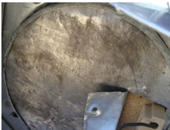
Figure 16. Bottom side of typical locally produced electric stove –Bottom of clay plate in contact with body of stove
