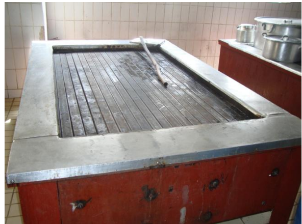
Figure 13. Locally manufactured “Karenbola” type electric stoves for large kitchens, 21 Kw
