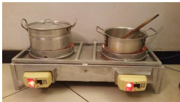
Figure 11. Double and Single stoves having bottom insulation and top lateral heat retainers
