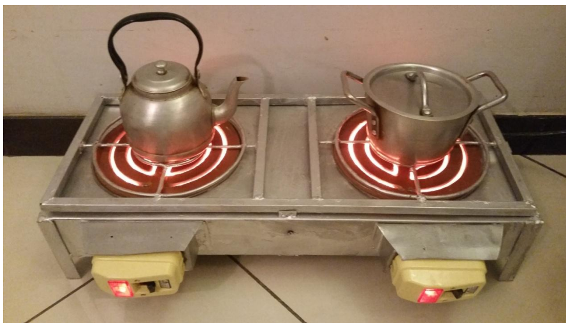
Figure 21. Typical mismatch between cookware base and stove tops
