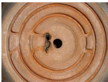
Figure 23. Effect of spillage and short circuit of resistance on clay plate of stoves
