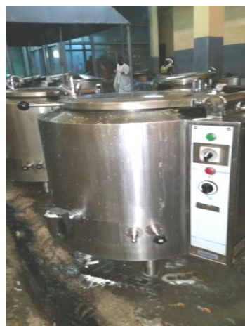
Figure 14. Imported electric powered, self contained, steam based cooking pots at Addis Ababa University, Main campus cafeteria
