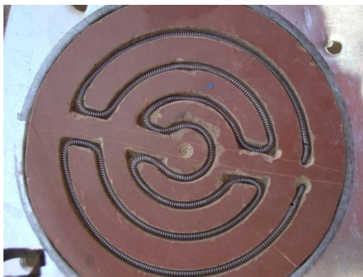
Figure 18. Groove and gap of cooking pot rest on local stoves.
