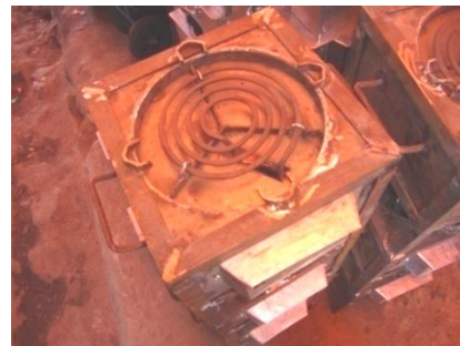
Figure 10. 22 cm single spiral hollow steel tube electric stove
